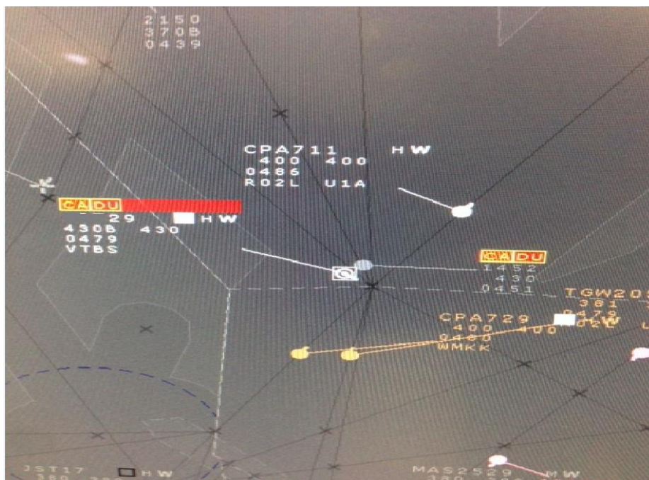
Fig 2: Automation system displaying DUP alerts
